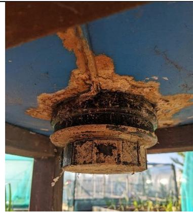
These are the three posts that I used for creating the pocket shape and holding it until it cools. They are 7.5cm diameter, I cut 1.6m posts in half at a roughly 45degree angle. This allows for easy insert to shape the pockets. Using three posts allows enough for the shaped pockets to have cooled and move the first used on to shape the next pocket.
