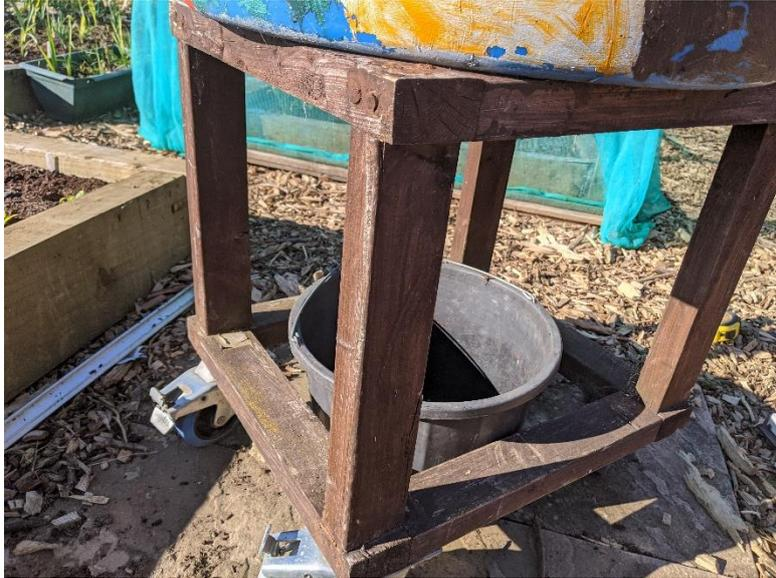
This is very simple to build. Just two rectangles 45x49cm made using 6x4cm timber anything close to this will be fine. The lengths of wood are all 45cm, the extra 4cm comes from the width of one length of timber. I screwed the timber together using 8 or 10mm screws having pre-drilled and counter sunk holes for the screws. The two rectangles are then screwed together using 4x35cm lengths of the same timber, one piece at each corner.
